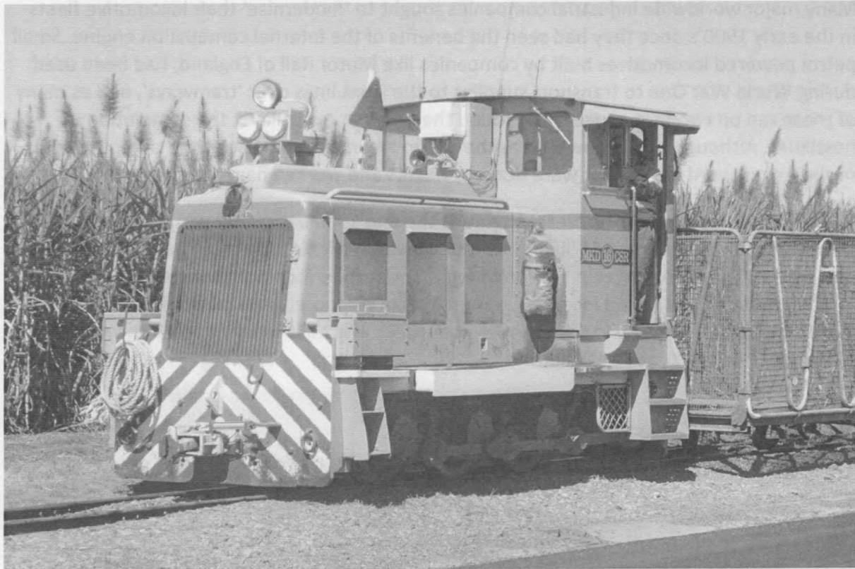
Macknade sugar mills No 16. The first Clyde built cane field locomotive.
