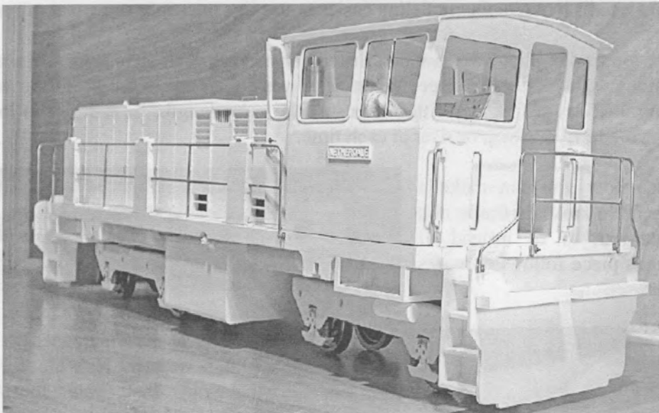
Loco's basic body 'box' shapes under construction (above and left column next page) with holes left for windows, louvres, etc.
