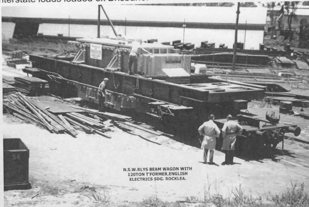
Transformer on Beam Wagon at G.E.C. Siding, Rocklea.
