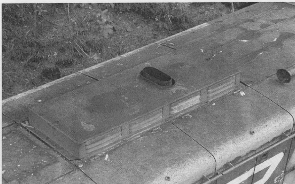
Square exhaust cover as fitted to 1738D & 1770D
