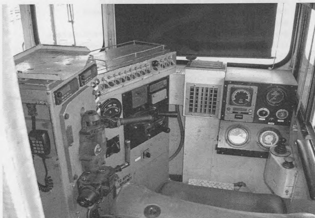
Control stand of 1734D showing rearranged control stand and 26L brake valves
