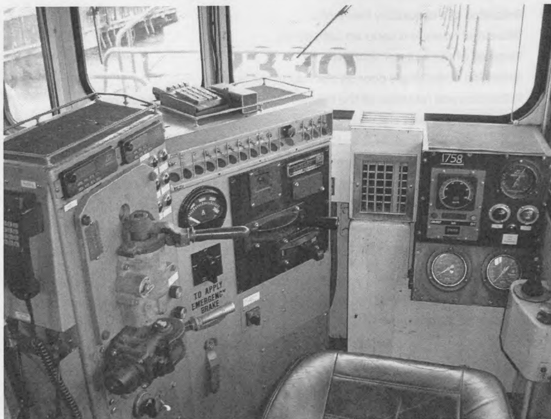
Control stand layout for the TSC 1720 class
