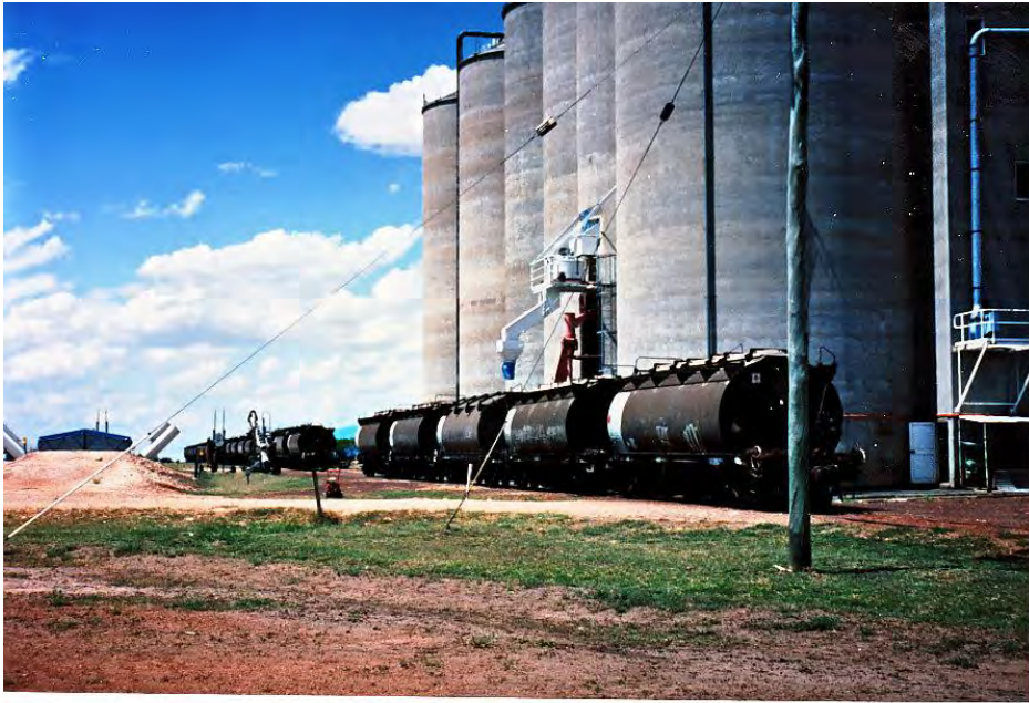
Hopper wagons with sliding roofs were gravity loaded with Bulk Wheat directly from Silos.
