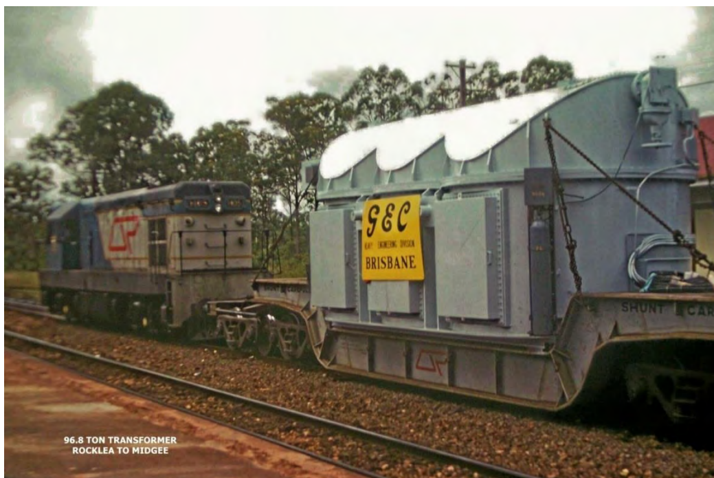
A 98.6 ton Transformer leaving GEC at Rocklea for Midgee.
