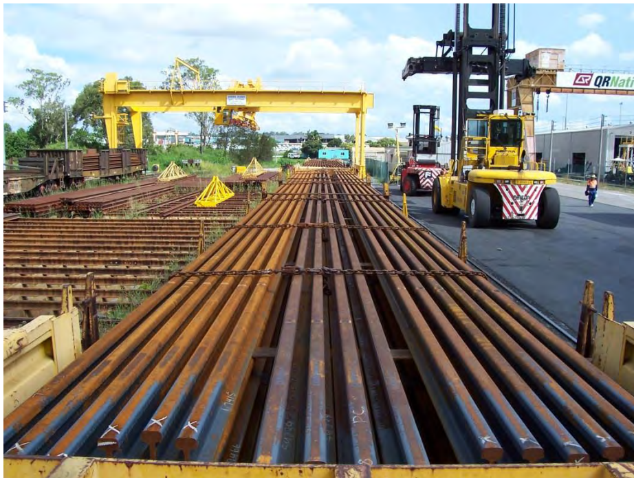
Chain secures the welded rails to the carrying wagons.
