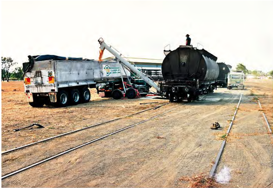
Mobile augers are also used for transshipment.
