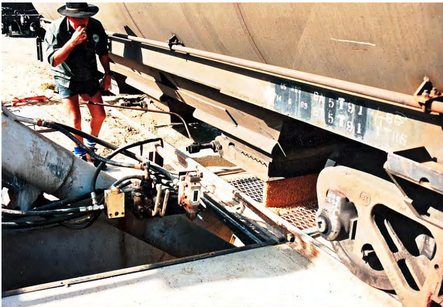
Bottom dump doors allow the Grain to be discharged into a pit where an auger takes it away to storage.
