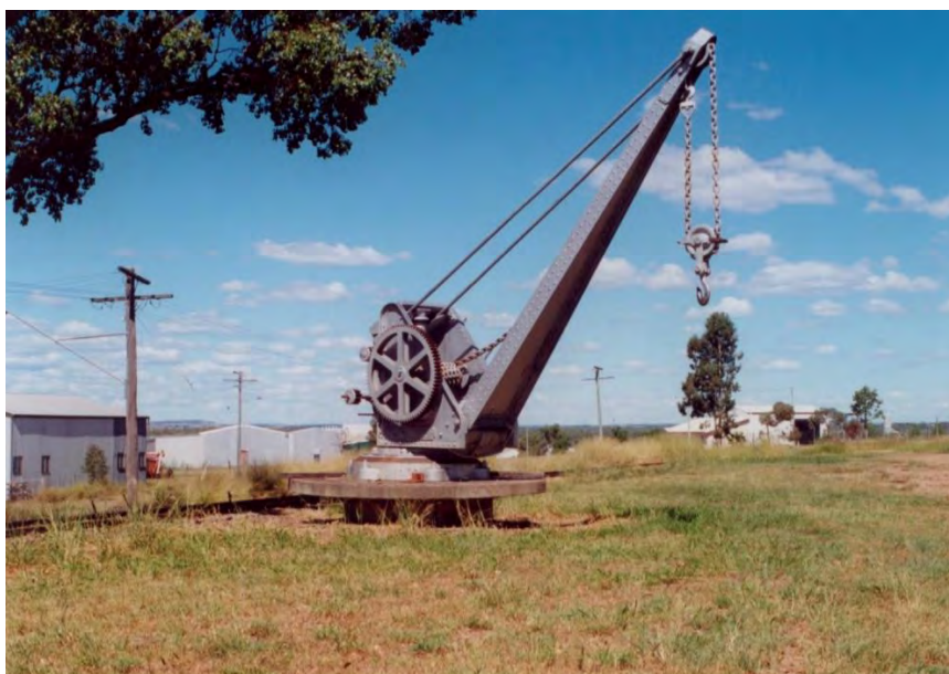
Wandoan used a Ten Ton Crane. All these Cranes were manually operated.
