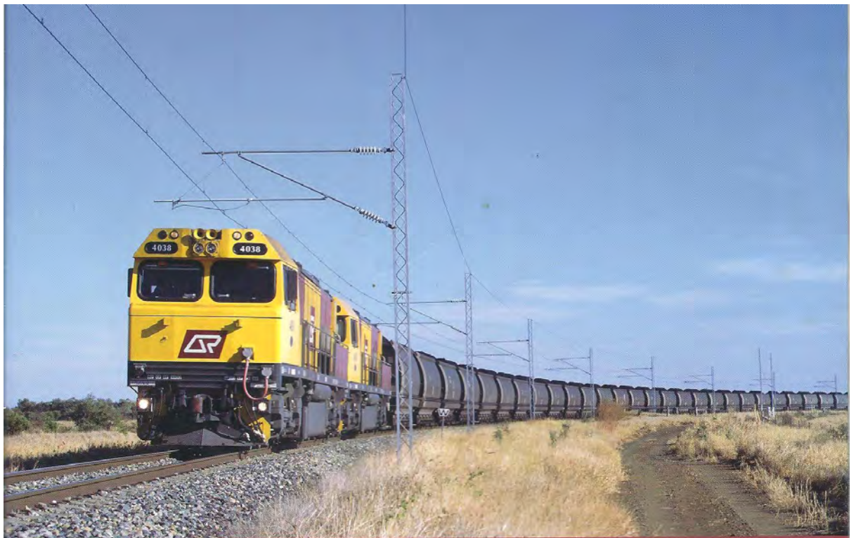
In the modern era, multiple Class 4000 DELs haul loaded aluminium coal hoppers towards a shipping port to load the coal for export.
