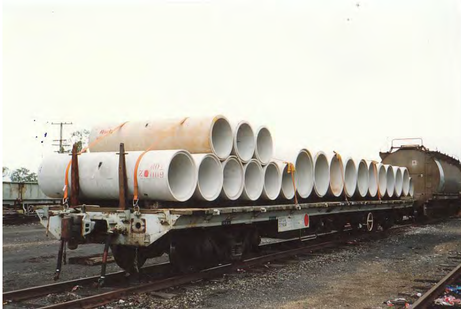
Concrete pipes for roadworks were carried on QFC wagons.
