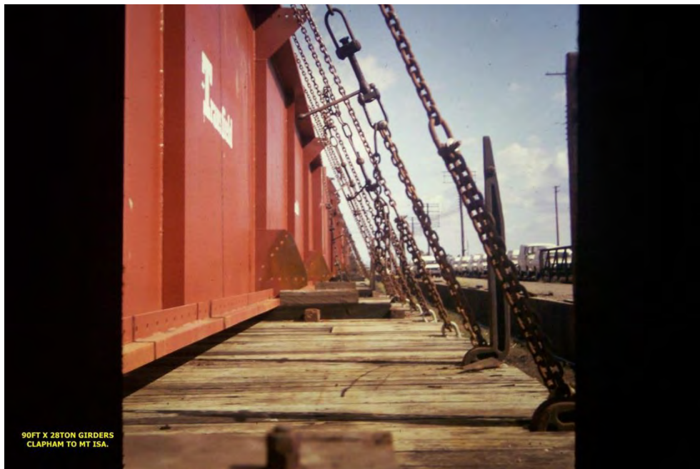
Chains secure a 90 foot long girder.
