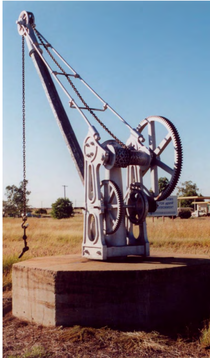
Muckadilla used this 3 Ton capacity Crane. Note the octagonal concrete base.
