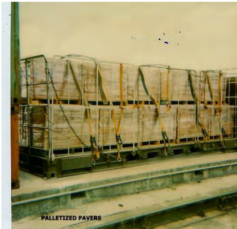
Concrete pavers were carried on pallets loaded by forklift.
