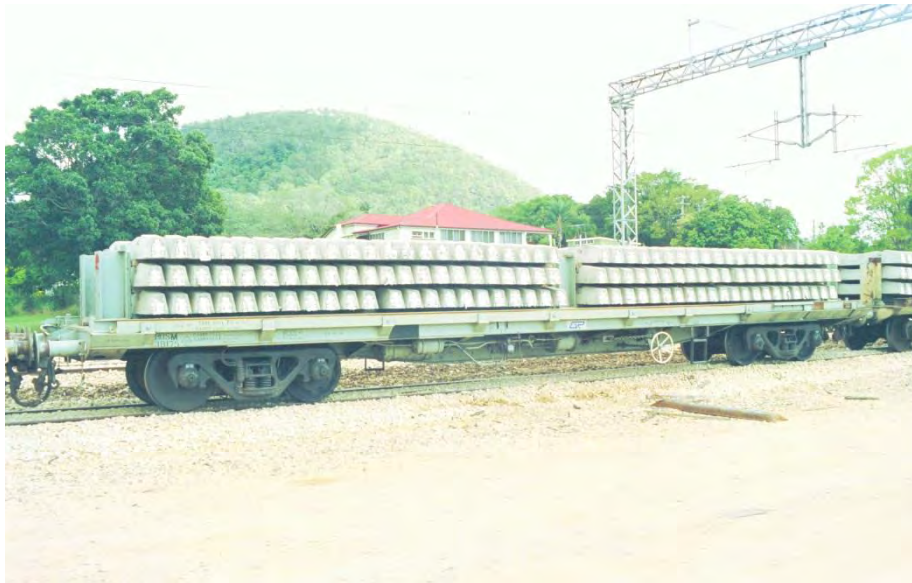
HOSM wagons carrying concrete sleepers at Beerburrum.
