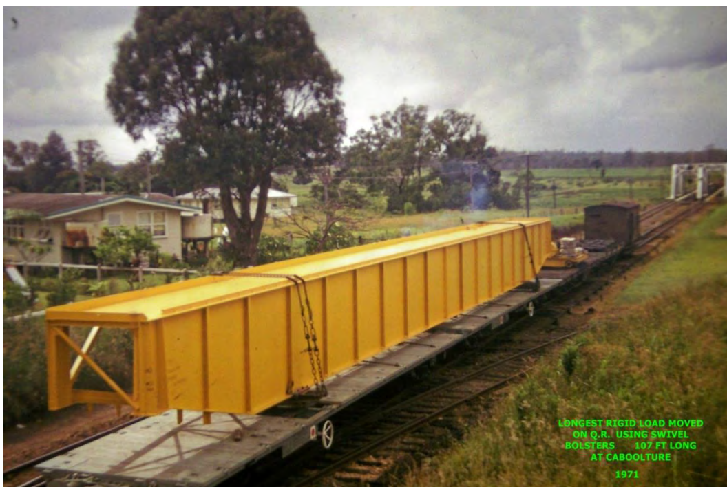
A 107 foot long Fabricated Girder is hauled to the North as a 'Special Load' on two wagons fitted with swivel bolsters.
