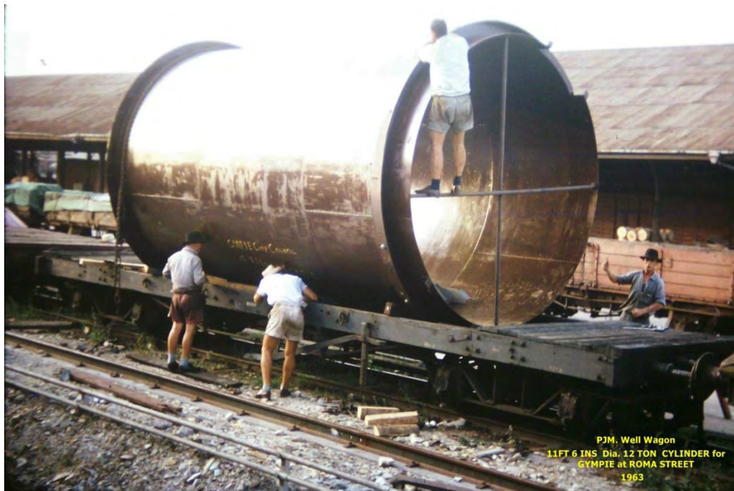
An 11 foot 6 inch diameter Ball Mill for mining at Gympie being loaded at Roma St onto a PJM well wagon. 1963.
