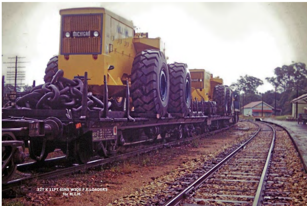
End Loaders which were 11 foot six inches wide on QFC wagons. Note the overhang of the wheels at the side of the wagon.
