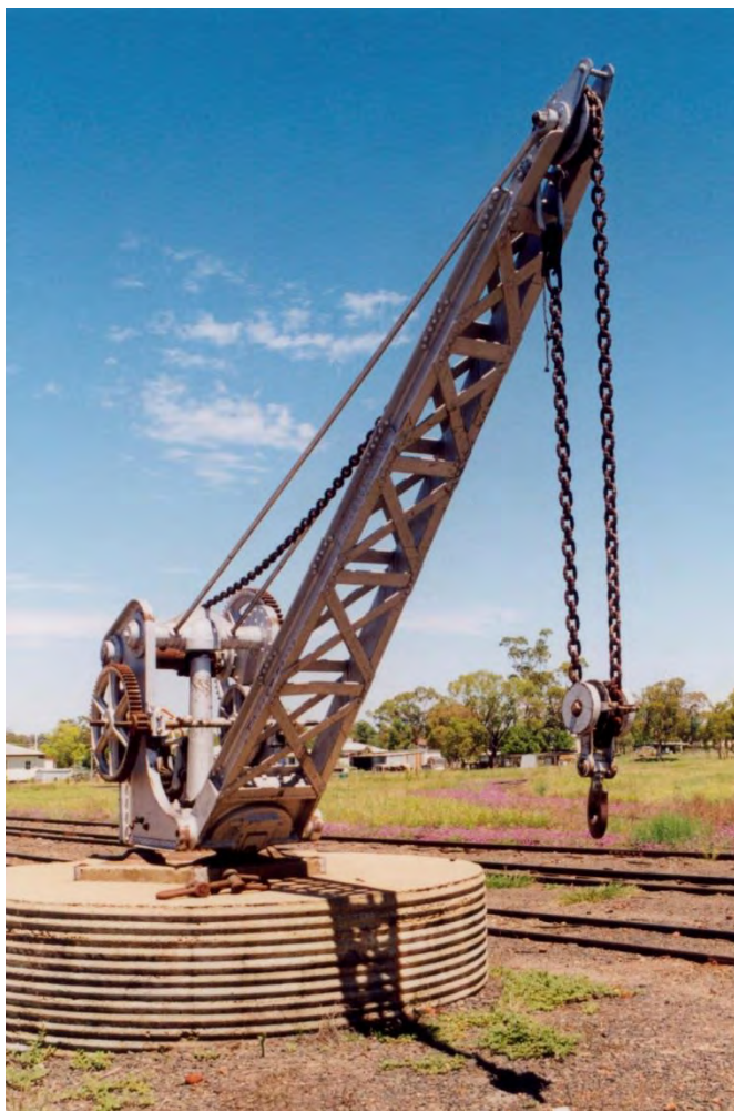
Morven had a Five Ton capacity Crane. A corrugated iron water tank was the former for the concrete base.
