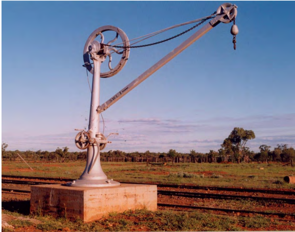
This One Ton capacity Crane is at Cheepie. The 'Whip' Cranes were a product of Ipswich Railway Workshops. They could be mounted on poured concrete bases or on a wooden loading platform.
