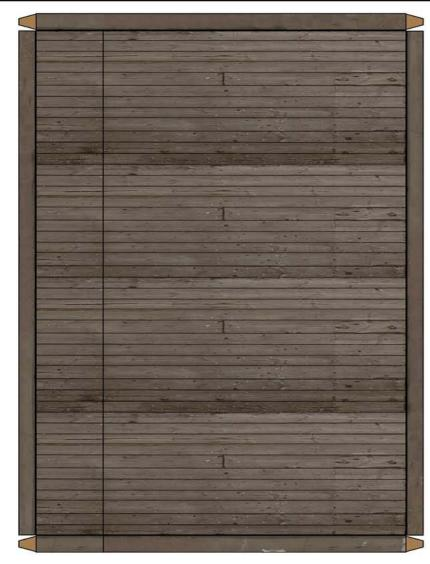
Assemble deck texture (above) first as a chocolate box lid, ensuring corners are square and edges vertical. Platform underside (stump base) folds and fits inside like box bottom, ensuring that it cannot be seen from side.
