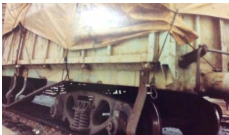
HSA (notice angle corner under doors)
