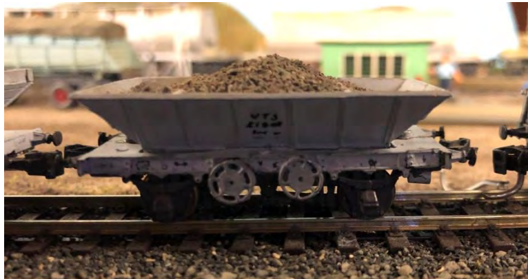
VTS scratch built by Arthur Hayes in the 1970s using Peco Underframes
