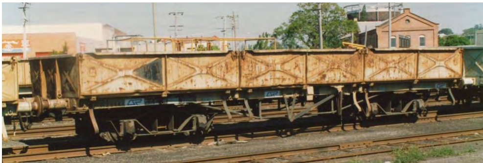
HJS 29444 with 2ft 2in Arch Bar bogies North Ipswich 10-1989 - KMCD
