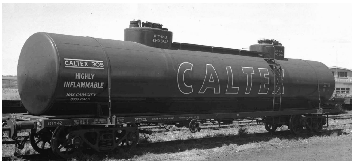
OTY 42 (AMRA Qld Library) Only wagon to be fitted with QR 10 Bogies.
