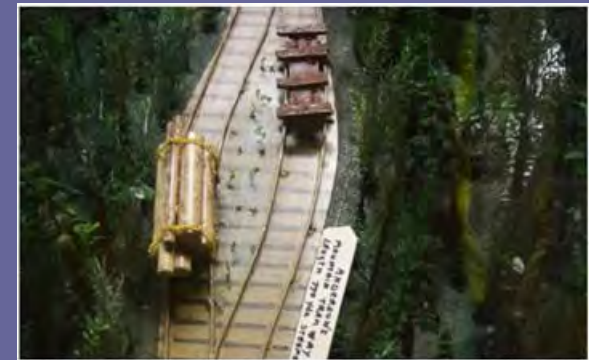
The tramway worked on gravity ... as logs rolled down the tracks, an empty carriage was pulled back to the summit
