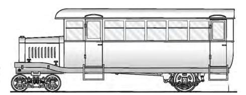
Douglas Shire Tramway rail bus built by PDST engineers. Jim Fainges provisional drawing from photographs.
