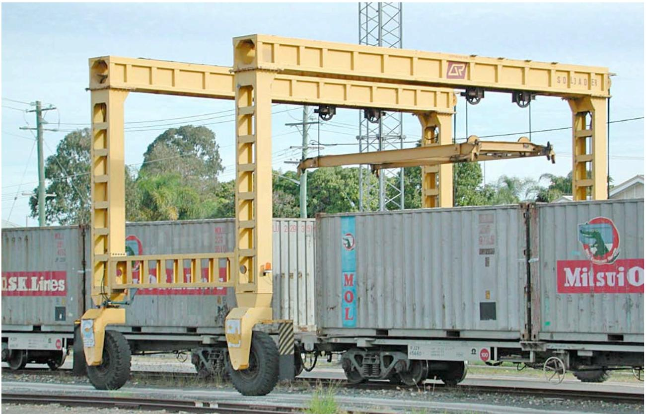
ISO standard container handling crane (above and bottom previous page) for transferring containers to/from rail/road transport, Bundaberg 2003. Lynn Zelmer photo.
