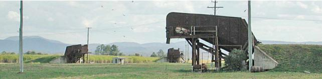
These loading ramps still existed near the old Wallaville mill in 2002 (to the right of the shed in the photo on page 1). They were used to transfer cane from road transport to cane bins for handling in the mill and consist of the ramp itself and a conveyor to raise the cane over the empty bins waiting on the track below. With ramps on either side of the open area to service cane arriving from either direction, it's obvious that the mill yard covered the whole area between. Lynn Zelmer photo.
