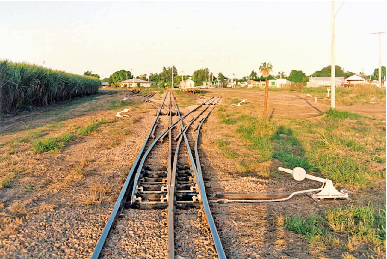
Dual gauge track and points at Kalamia Mill's Town Terminus at Ayr.
