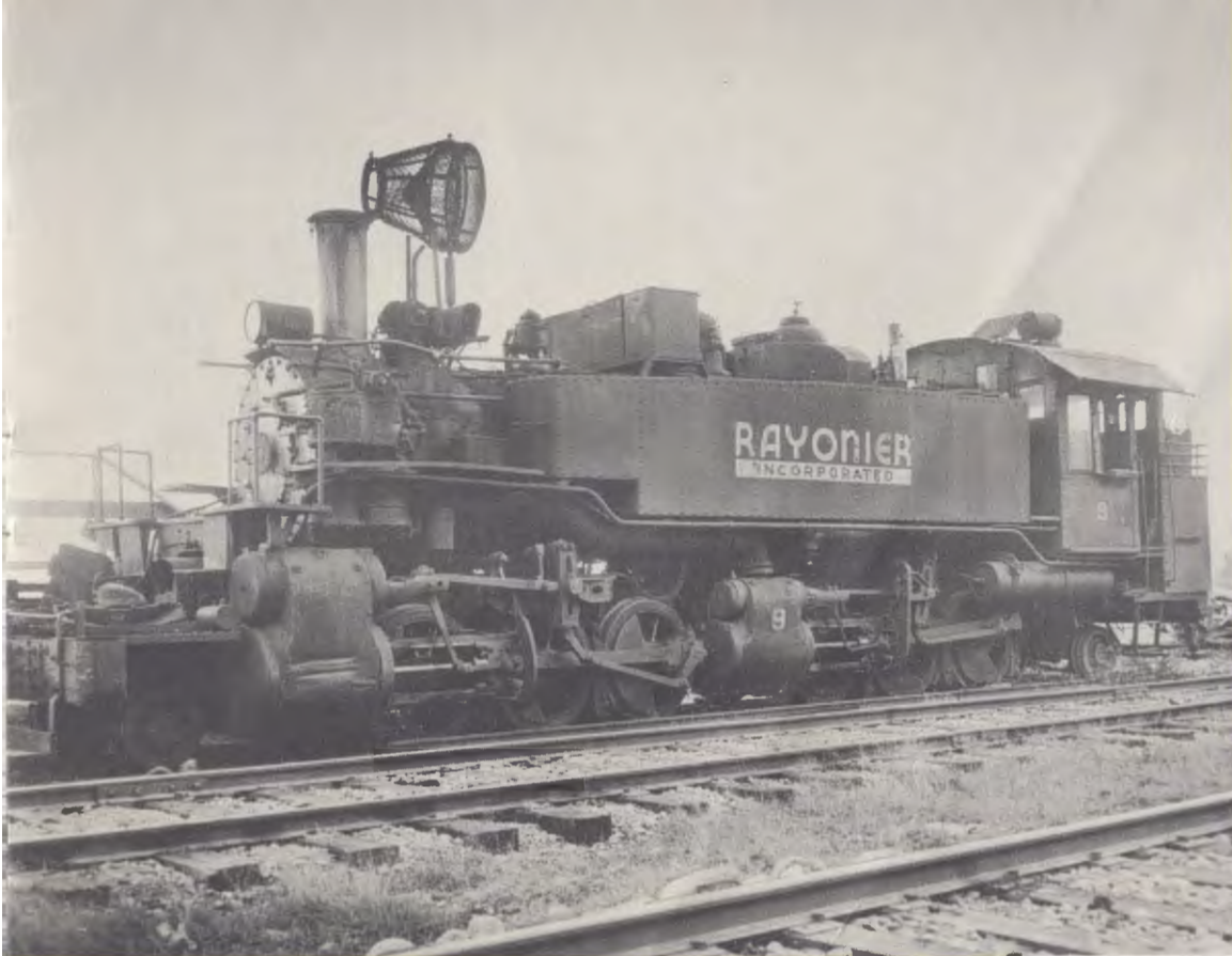
This is a 110-ton Baldwin "side tank" Mallet engine. Note the water tanks built alongside the boiler. This added weight over the drivers gave the engine additional traction. These side tanks also eliminated the need for a locomotive tender.
